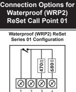
Option 1 terminals 1 & 2 Normally open switch closing on alarm
