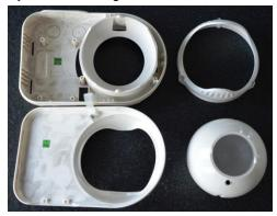
4. Use a screwdriver to open the two halves of the eyeball.
