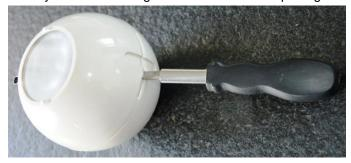
5. When open, remove the top half and note the battery connector.
