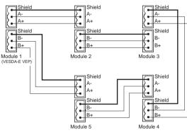
The diagram shows an example of the wiring for a closed VESDAnet loop, which is the recommended configuration. Remove the factory default A and B links from the VESDAnet sockets (C and D) prior to connecting the detector to the VESDAnet. It is recommended that 120 Ohm twisted pair cables (e.g. Belden 9841) be used for including the devices in the network, with a maximum length between devices of 1.2 km The polarity of the data wires must be maintained throughout the network.
