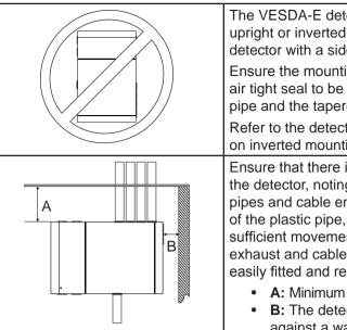
The VESDA-E detector can be mounted in an upright or inverted position. Do not mount the detector with a sideways orientation.
