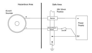
Fig 5 Single stage alarm using two channel barrier.
