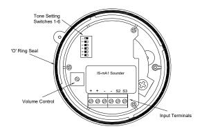
Fig 2 Location of field terminals and controls.
