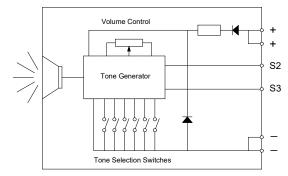
Fig 1 Simplified block diagram
