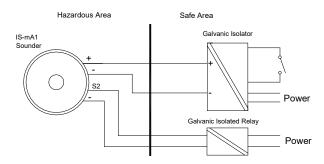
Fig 8 Multi stage alarm using galvanic isolated relays
