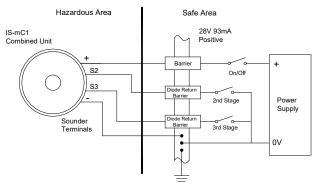
Fig 6 Sounder multi stage alarm using Zener barriers.
