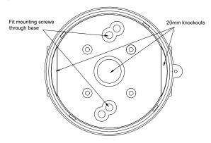
Fig 3 Mounting Combined Unit Base.
