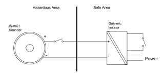
Fig 9 Sounder single stage alarm using galvanic isolator.
